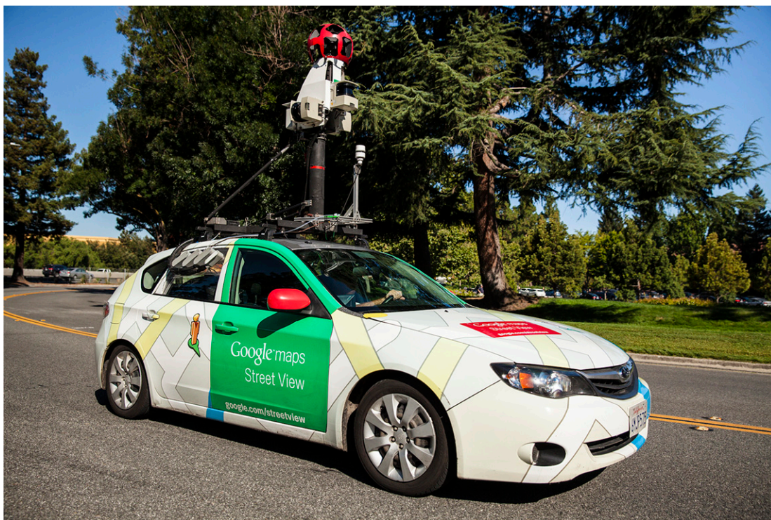
Google isn't only driving through neighborhoods to update its maps. This car, equipped with an air pollutant sensor, traveled through the streets of Oakland in 2014 and 2015 to get detailed readings of nitric oxide, nitrogen dioxide, and black carbon particles. Image courtesy of Aclima/Google.
